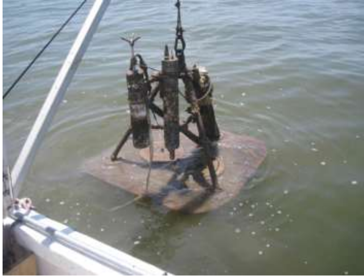
Fig. 5.2. ADV being retrieved for monthly data acquisition and maintenance.
