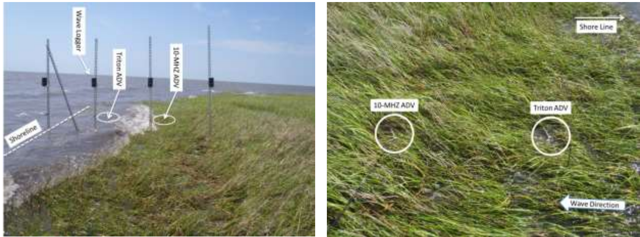
Fig. 3.25. Schematic drawing of instruments deployment setup. Left: Wave logger; Right: ADVs
