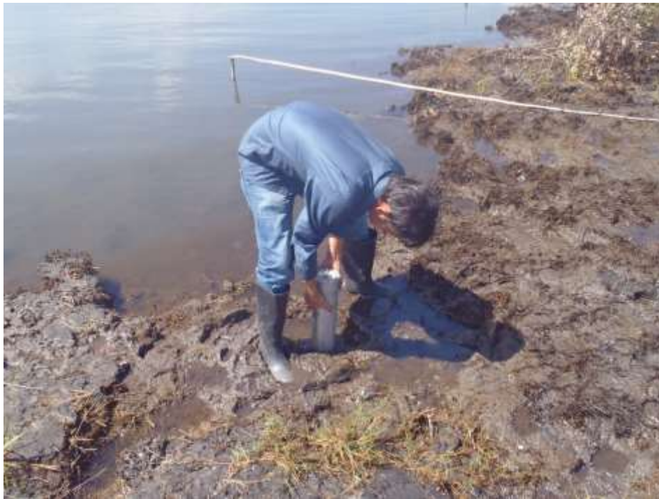
Fig. 4.32. Undisturbed sampling with a vibracore aluminum tube
