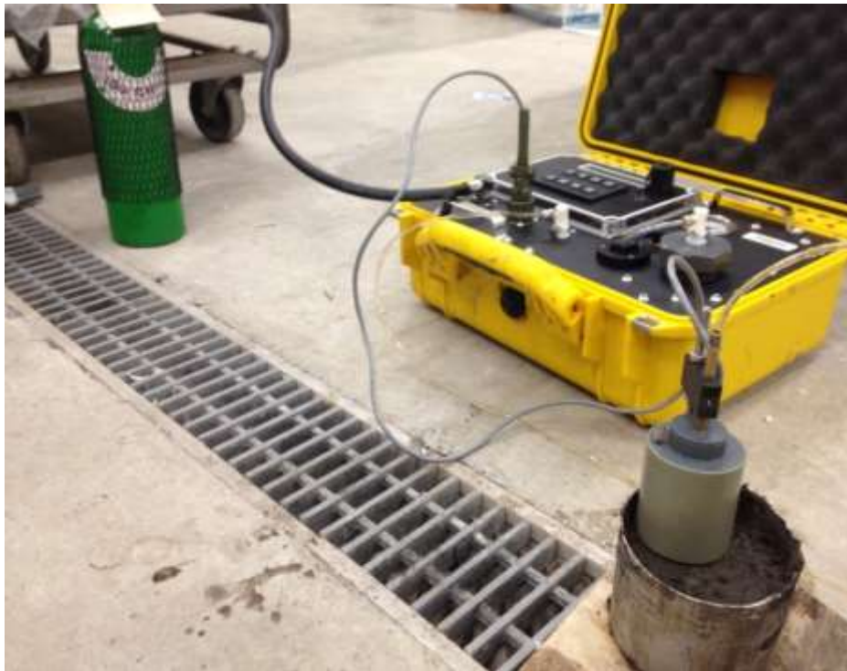
Fig. 4.33. Running cohesive strength meter test on small 3 inch soil sample tube
