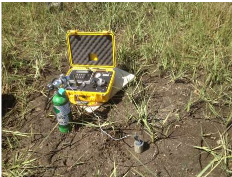
Fig. 4.31. An in-situ CSM test being performed in the Terrebonne Bay site.
