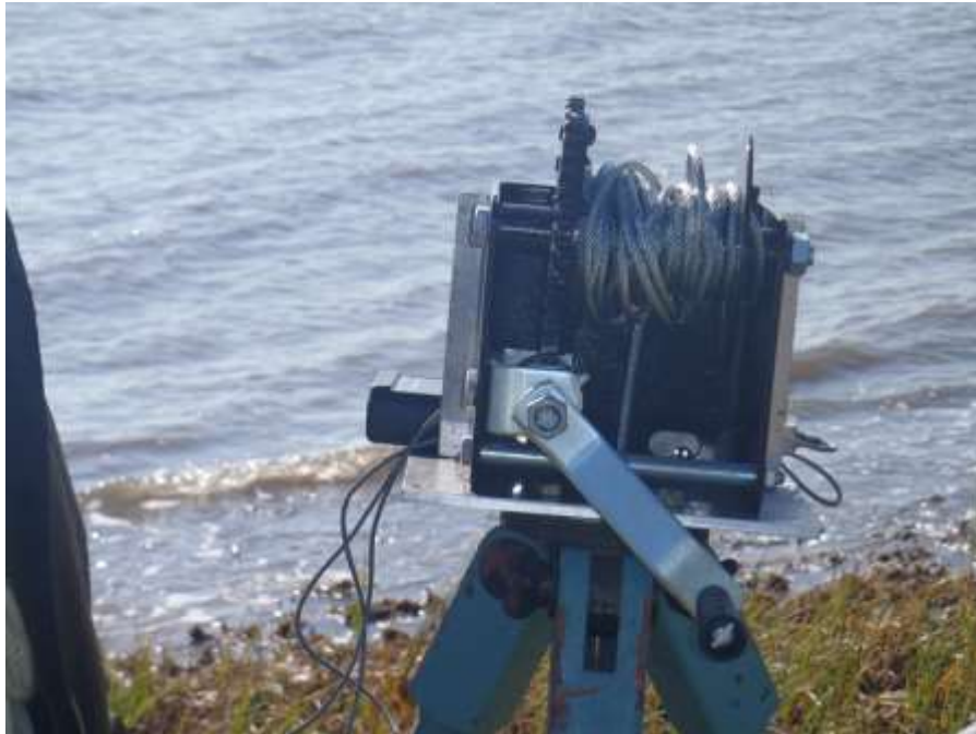
Fig. 4.8. A worm geared winch connected to aluminum mounting bracket atop the tripod.
