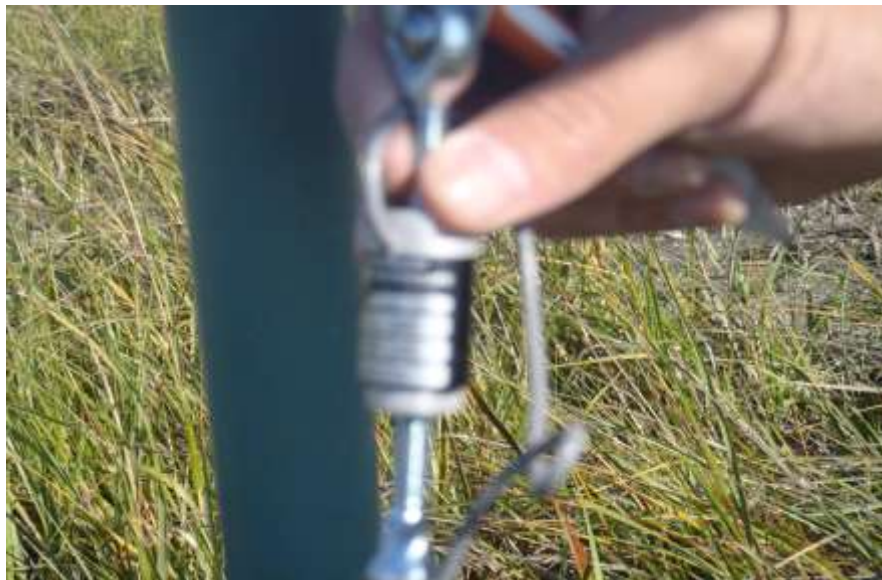
Fig. 4.9. Photograph of in-line tension load cell.
