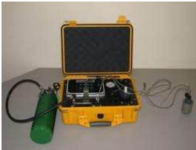
Fig. 4.29. The cohesive strength meter connected to a compressed air tank and the cylindrical sensor head
